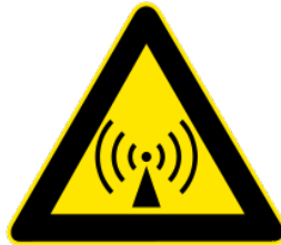
Figure 2: Warning sign for radio-frequency non-ionising radiation
